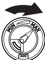
Clockwise to reduce water drops and hard water spots
