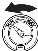
Counterclockwise to reduce foaming
